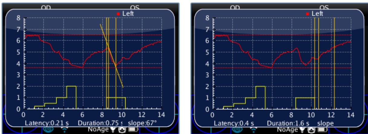
By pressing the EYE (Button D) button in the 2WIN, the system of four lines will be displayed on the following event of transition in the pupil diameter. Then if the EYE button is pressed again the overall measurement procedure will be started in the DX eye.
