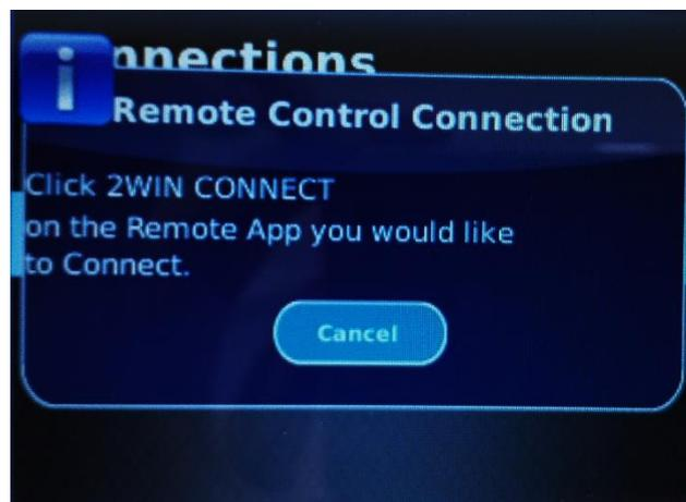
6. From the tablet Application open the Settings panel and select 2WIN Connection
