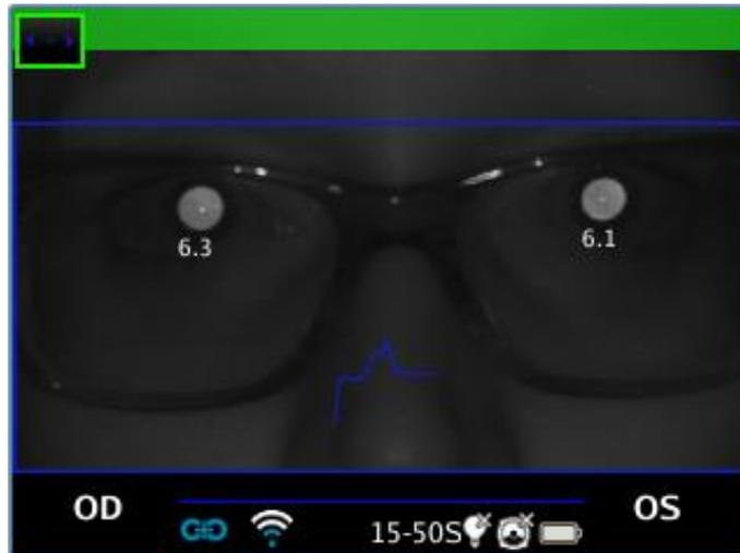
After the measurement is done, the main PD information is displayed at the top of the Application's main display.
