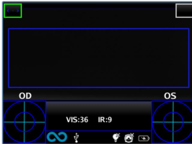
**Good light conditions are equivalent to a value of VIS between 30 and 80, and of IR less than 30.**
