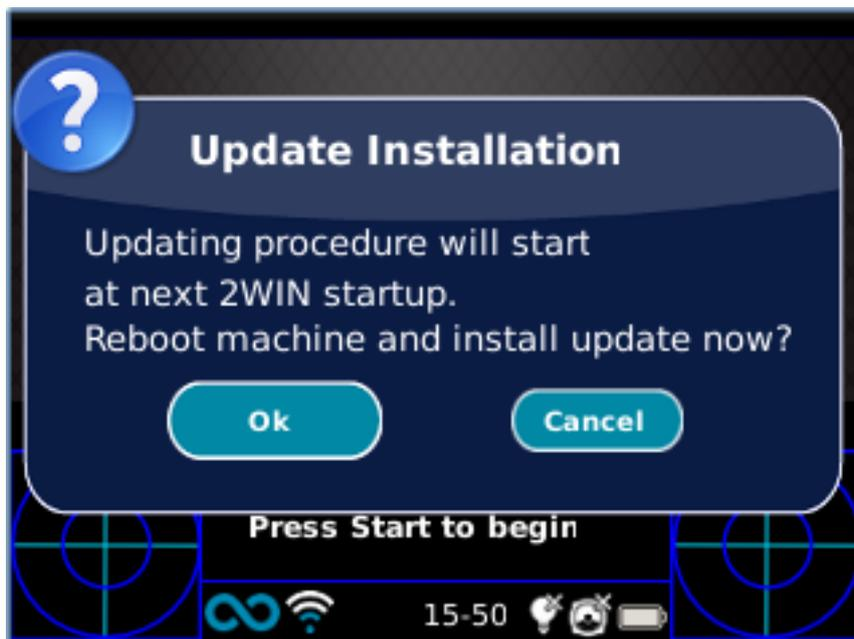
After the extraction file, 2WIN will prompts the request of immediate or delayed installation. If OK button is pressed, 2WIN will restart and run the system update. Press the CANCEL button to delay the update (the update will take place at next 2WIN reboot). System update will start at next startup.
