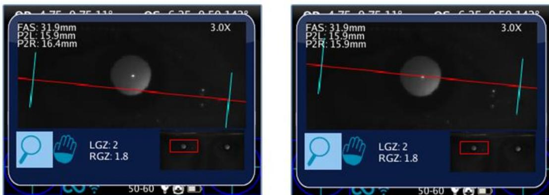
Press MENU again to select left and right vertical axes and move them with MENU\_LEFT and MENU\_RIGHT. Pressing MENU again to go out of axes selection and to change eye or modify zoom factor.
