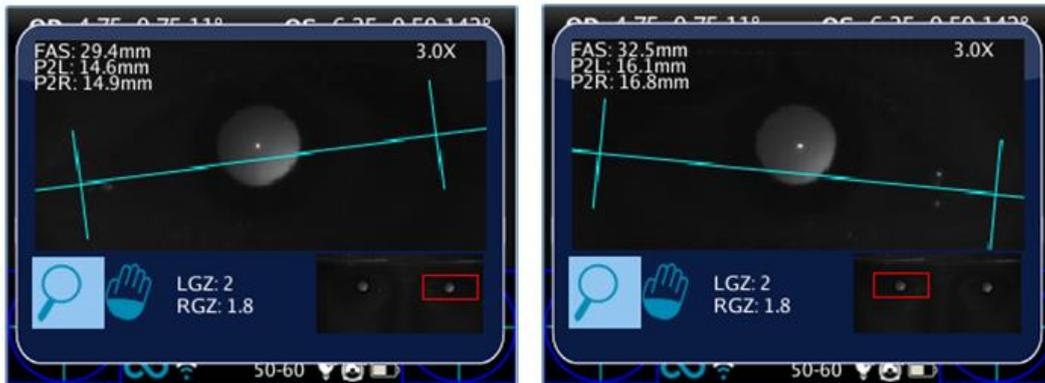
With MENU key it is possible to change axis to set its position. First pression to move horizontal axis: when selected the button shifts it up and down with MENU\_UP and MENU\_DOWN, MENU\_LEFT and MENU\_RIGHT change inclination to match real eye position.
