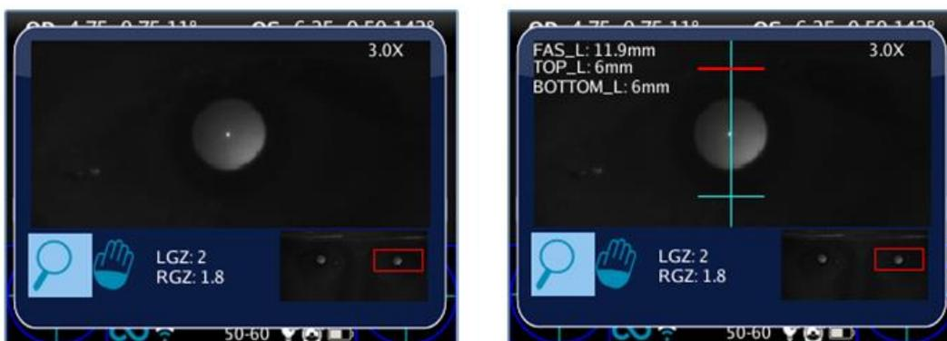
Press EYE key to enable Eye Morphology functionality when in zoom mode: first pression for vertical mode measurements, second pression to get horizontal mode.
